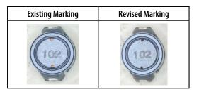
The form of the affected part numbers will change slightly due to the change in the marking process. The fit and function of the affected part numbers will remain the same. The quality and reliability of the affected part numbers should be improved as a result of the change to automated manufacturing processes.
